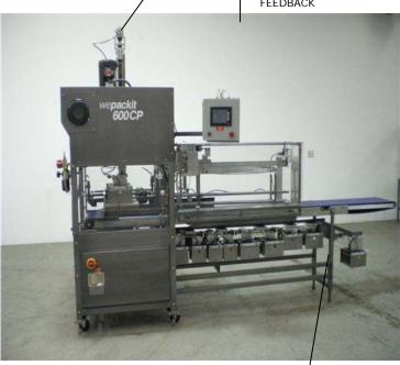
2" TUBULAR WELDED CONSTRUCTION 'CLOSED BOX DESIGN'
