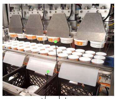
locator guides, secure dairy or corrugate cases, permitting unobstructed product entry head end-effector secures containers and collapse rows for nested pack patterns
